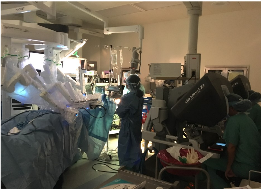
Fig. 5 Nurse views procedure on screen while resident observes through da Vinci console (right). Patient cart (left) is attached to patient.
