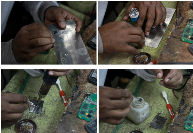
Figure 3: Steps of Reballing (clockwise, from top-left): Placing IC on the net, Applying liquid metal to fill up the ball gaps, Applying soldering paste and hot air to melt and place metal nicely on the IC, Cleaning the IC .
