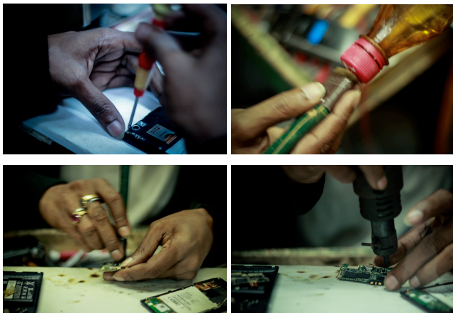
Figure 1: steps of servicing (clockwise, from top-left): opening the back-cover, putting thinner on brush, brushing the motherboard, blowing hot air.
